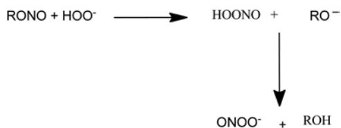
Scheme 3.2 Peroxynitrite synthesis via the reaction of hydroperoxide anion and alkyl nitrites.
